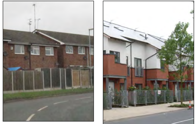
Fig 5.10 New dwellings must overlook streets and spaces both within and around the development. Backs onto surrounding streets (left) should be avoided.
