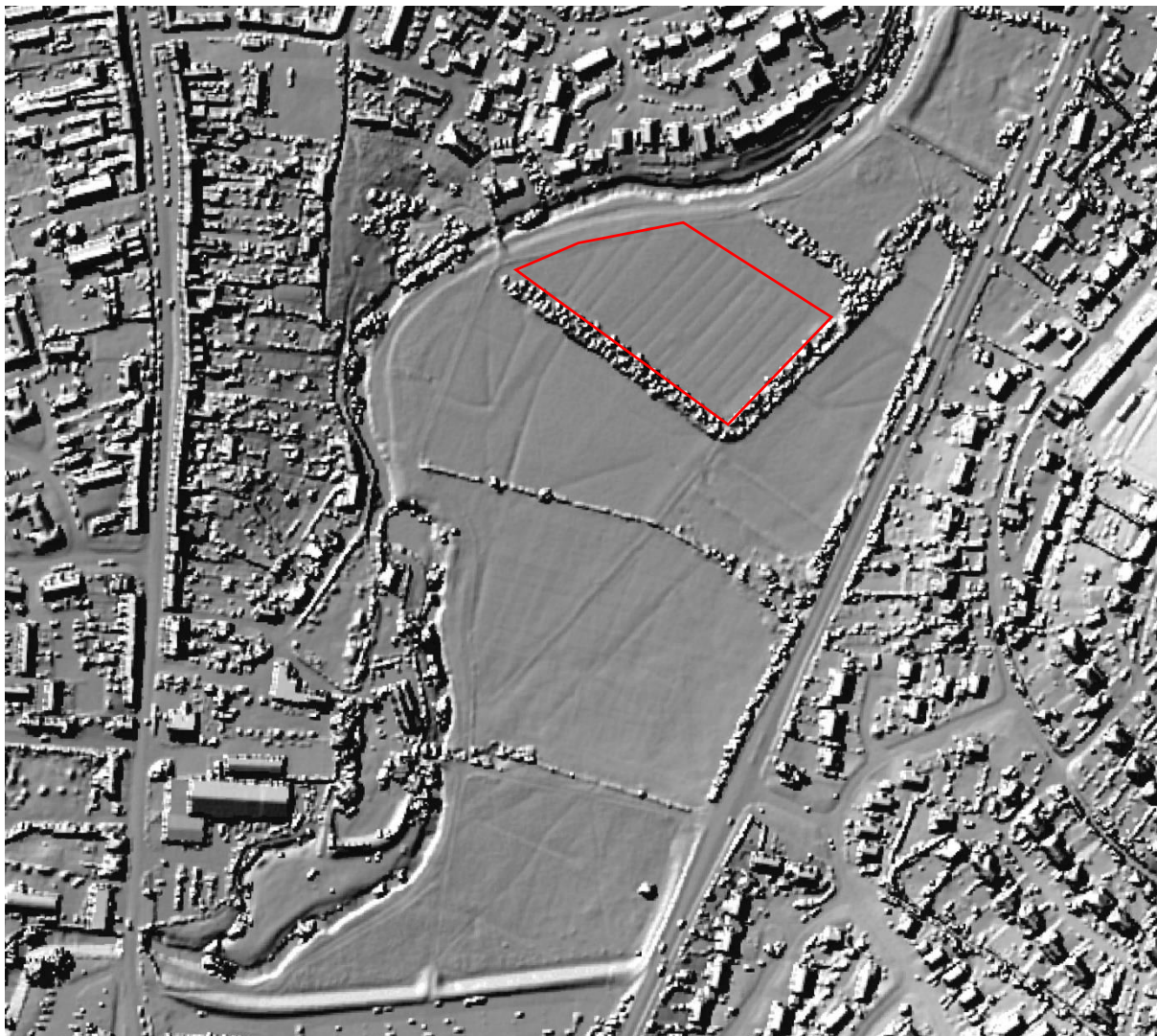
Figure 5: 1m resolution LIDAR data, with the area bounded by the red box containing parallel lines (former drainage ditches?) possibly indicative of a former water meadow, though no main or tail drains are apparent.
